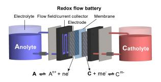
and its capacity can be scaled up just by increasing the volume of the tanks. The electrolytes flow through an electrochemical cell where redox reactions happen. Due to this design, one of the distinct features of RFBs is the decoupling of their energy storage and power generation. Thus, they are suited for grid-scale energy storage up to MWh.
